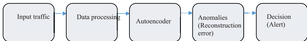
Figure 2. Description of the operation of an autoencoder for anomaly detection in network traffic
